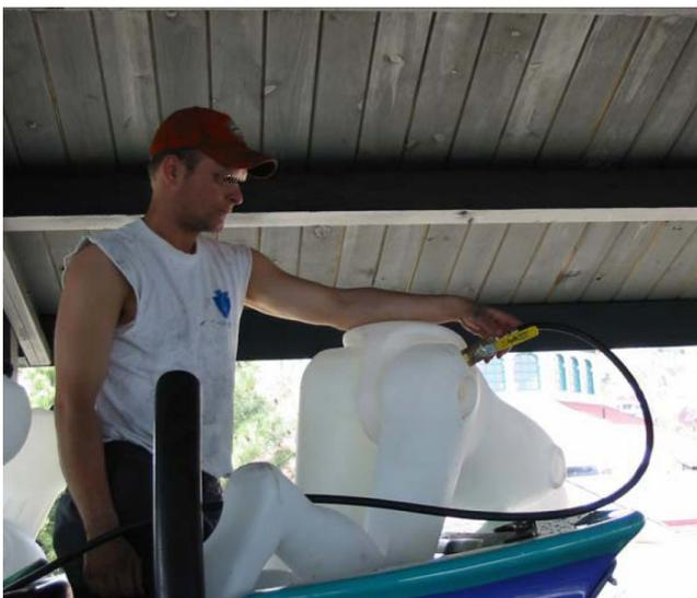
Fill torso/head portion of the dummy while it is in the ride seat. Be sure to turn all of the caps tightly. It is recommended that you twist these closed all the way by using pliers or wrench, especially at the waist so that it does not rub against the lap bar.
